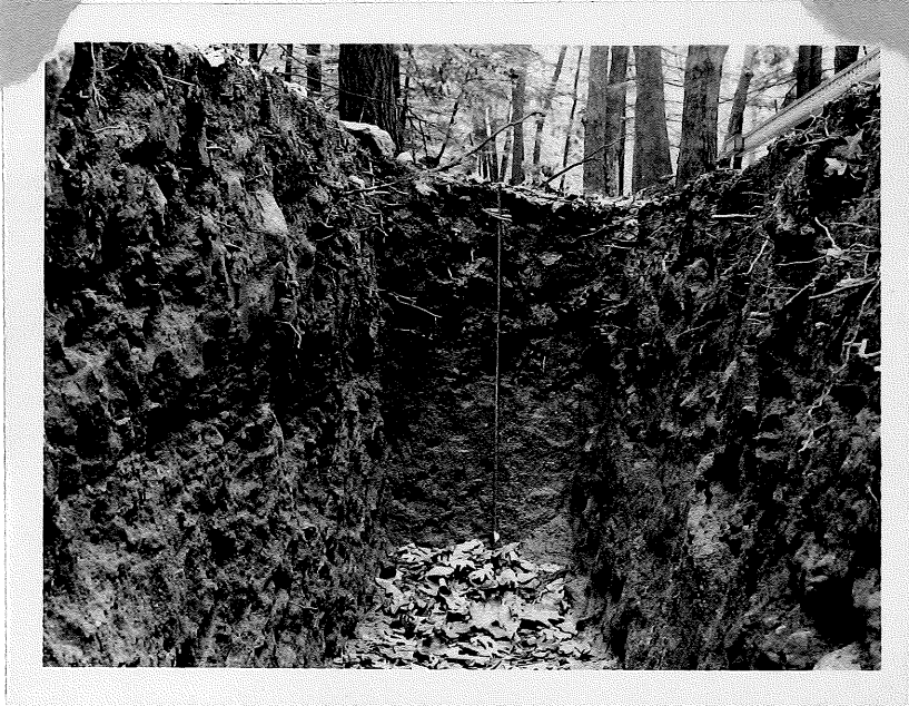
Fig. M-H-23, mound and pit No. 25. Knife at end of excavation marks upper surface of till. Till surface is practically horizontal and uniform on the left wall which is beyond the general regions of disturbance. On the right wall, which is within the disturbed regions, the surface of the till is irregular and has a perceptible dip.
