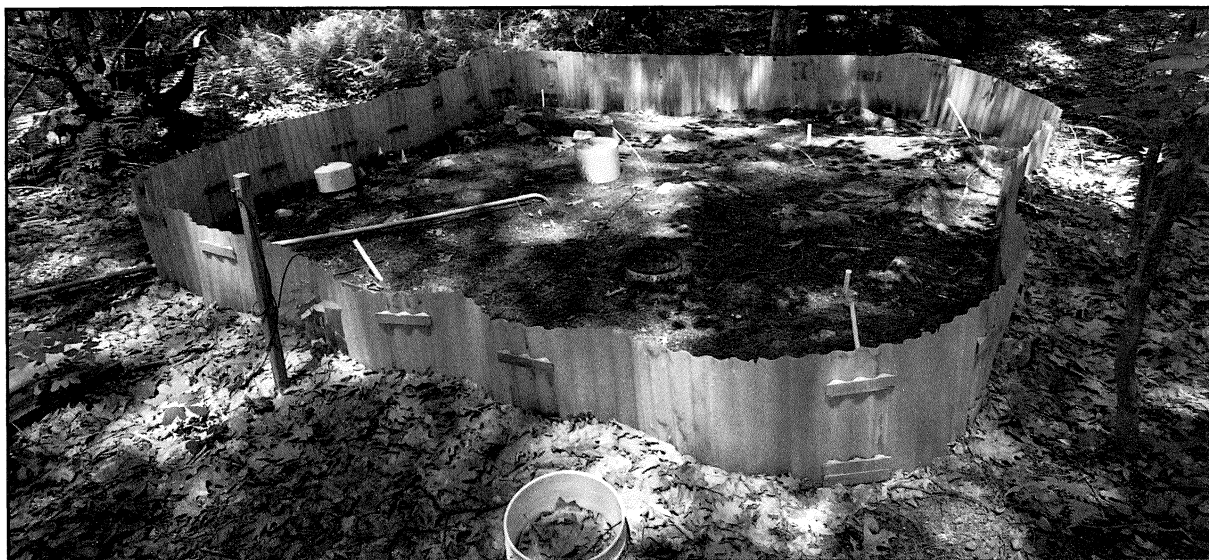
Detritus Input Removal Treatment (DIRT) Experiment. Manipulation of above- and below-ground organic inputs provides insights into the fundamental processes of carbon dynamics in forest ecosystems.
