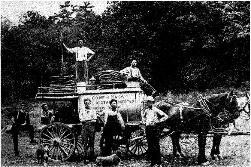
Our new power sprayer complete. This outfit was planned and built by the State Forester's department. Four-cylinder engine, triplex bronze pump, 300 pounds pressure capacity, weight 3,000 pounds. (Illustration from the Eighth Annual Report of the State Forester, 1911.)
