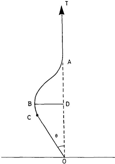
Fig. 2. A diagrammatic representation of a leaning *Pinus resinosa* tree in the process of vertical reorientation. O, ground level;  $\theta$ , angle of displacement of the bole from the vertical; A, point of correction of the displaced bole; BD, maximum horizontal displacement of the bole on the horizontal plane; C, end of the lower bole leaning leeward; T, tree top; AT, recovered portion of the tree.
