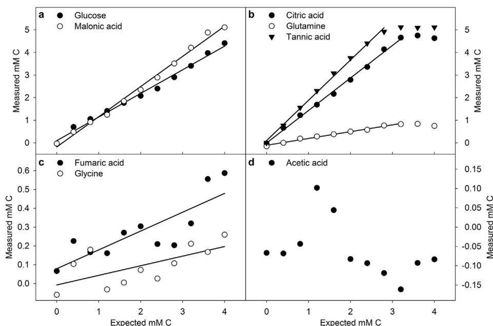
**Fig. 1.** Linear relationship between measured and expected C concentrations of eight common organic compounds estimated using a calibration curve based on oxalic acid. Regression coefficients and statistics are presented in Table 1. Only regressions statistically significant at  $P < 0.05$  are shown.
