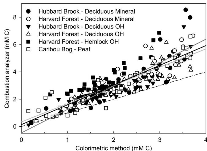
**Fig. 2.** Linear relationship between DOC concentration of soil extracts measured using the Mn(III)-pyrophosphate method and a TOC combustion analyzer. The regressions for OH and peat samples, MS samples, and all samples aggregated are shown as light gray, dark gray, and black solid lines, respectively. The dashed line represents the 1:1 slope. Regression coefficients and statistics are presented in Table 2.
