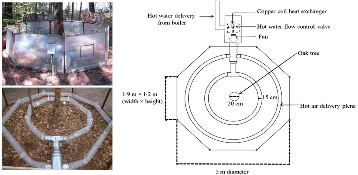
**Figure 2.** Warming chamber diagram, view from above. From Pelini et. al, 2011.
