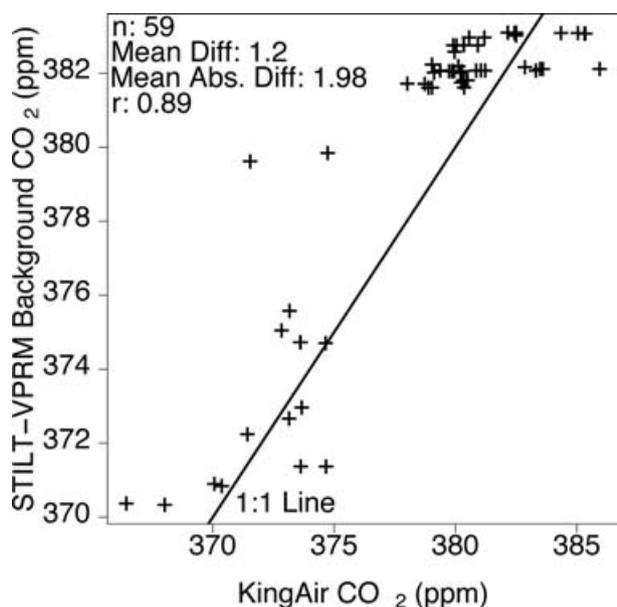
Fig. 9. Comparison of mean free troposphere CO<sub>2</sub> concentration determined from COBRA-Maine airborne observations and corresponding background value at Argyle tower, determined from the advected boundary condition in the receptor-oriented model (Section 2.2). Each point represents one aircraft profile within 50 km of Argyle.
