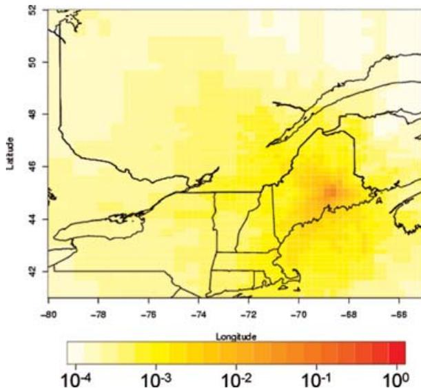
Fig. 4. Visualization of the average 5 d footprint ( $\langle\langle f \rangle\rangle$ , see eq. 2) for Argyle tower for daytime hours during the period 15 May to 15 September 2004. For each hour,  $\langle\langle f \rangle\rangle$  is calculated by taking the footprint function and integrating over all areas and all times for 5 d upstream, and the mean result is shown. Values less than  $10^{-5}$  are not coloured.
