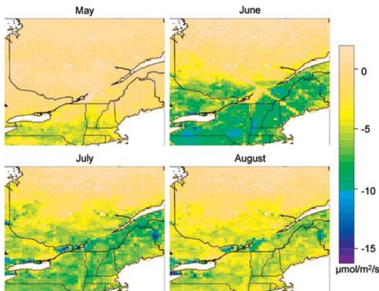
Fig. 5. Initially calibrated VPRM calculated mean monthly (all hours) fluxes for May (a), June (b), July (c) and August (d) 2004 in  $\mu\text{mol}/\text{m}^2/\text{s}$ , based on hourly calculations.
