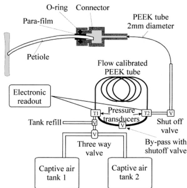
**Figure 1.** Schematic representation of the two-point flow meter. Water flows from one of two pressurized air tanks, through a tube of known conductance, and into the distal end of the petiole. The pressure drop across the calibrated PEEK tubing is used to determine the flow rate, while the downstream pressure transducer gives the delivery pressure into the petiole. Consecutive measurements of flow rate at two different pressures are used to calculate petiole conductance.
